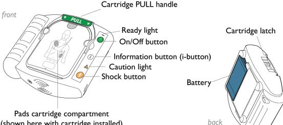
(shown here with cartridge installed)
